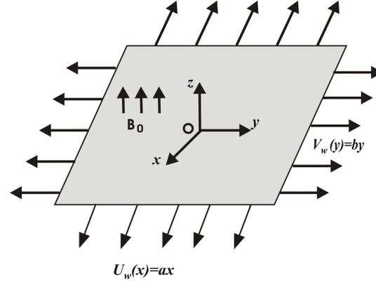
Figure 1: Schematic representation of the flow problem.
