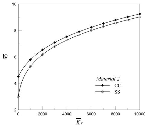
Fig. 4. Effect of boundary condition on natural frequency of FGM beam
