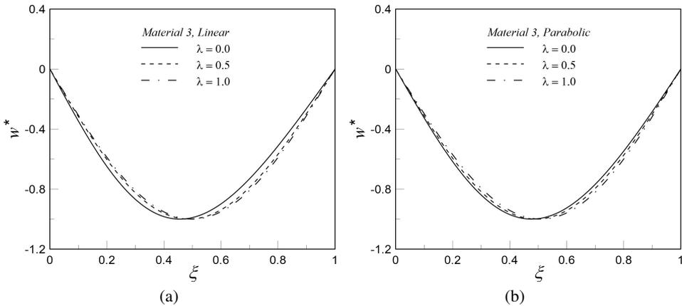
Fig. 7. Effect of foundation stiffness parameter ( $\lambda$ ) on the mode shapes of SS FGM beam (a) *Linear* (b) *Parabolic*
