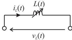
Fig. 9. Model of a coil of LTV class
