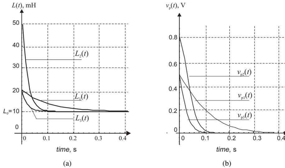
Fig. 10. Parameters variability of LTV coil: varying inductance:  $L(t)$  (a); control voltage  $v_p(t)$  (b)
