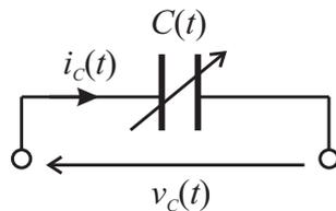
Fig. 5. Model of a LTV- class capacitor
