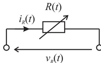
Fig. 3. Model of a LTV-class resistor
