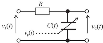
Fig. 7. Example realization of the low-pass LTV filter
