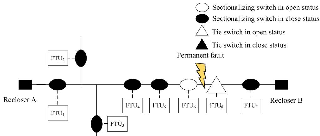
Fig. 3. The topological structure of the feeder shown in Figure 1 after the fault isolation
