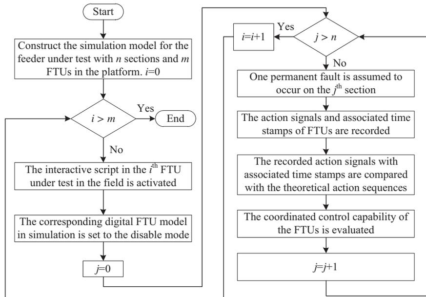
Fig. 5. The flow chart of the proposed cloud-based feeder automation testing method
