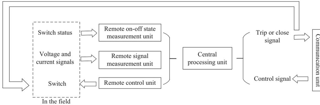
Fig. 8. The operating principle of the FTU in the field
