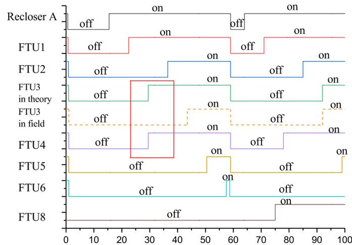
Fig. 11. The sequence diagram of the status of switches in the experiment (FTU3 is under test)
