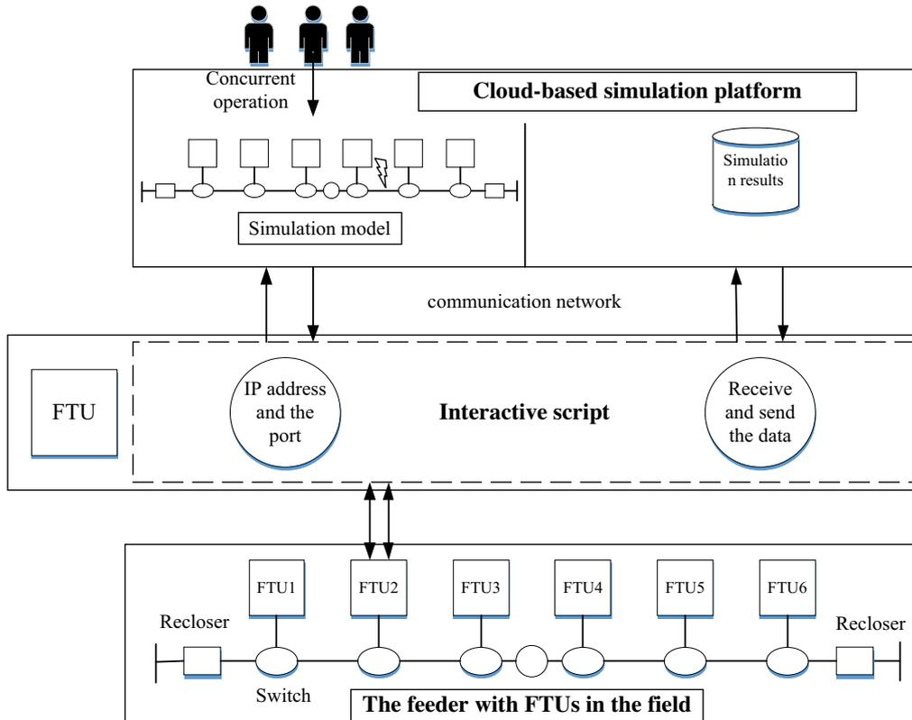
Fig. 4. The scheme of the proposed cloud-based feeder automation testing method
