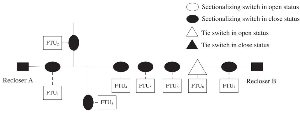
Fig. 1. A single-line diagram of typical ring main feeder with local-reclosing FA system
