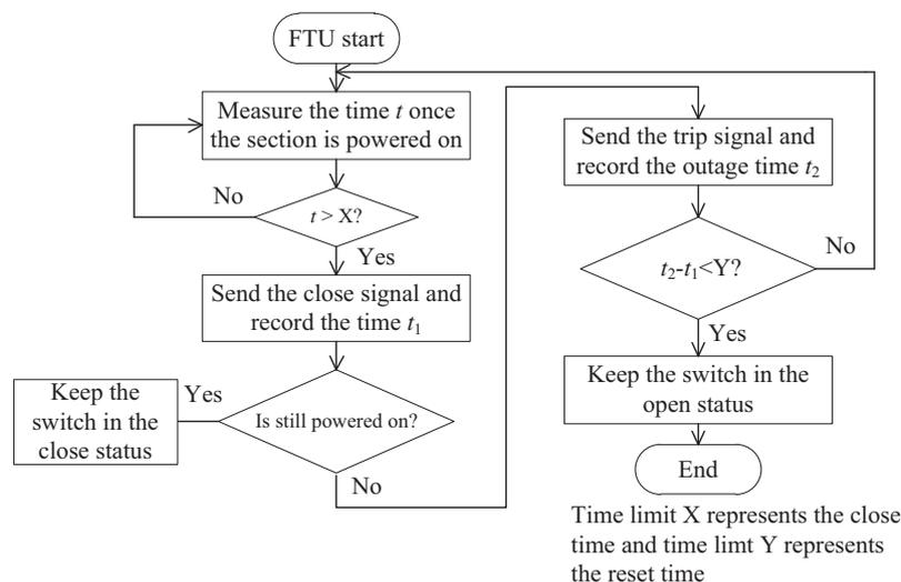
Fig. 6. The work flow of the FTU model constructed on the cloud-based simulation platform
