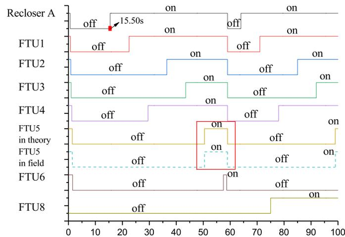
Fig. 10. The sequence diagram of the status of switches in the experiment (FTU<sub>5</sub> is under test)
