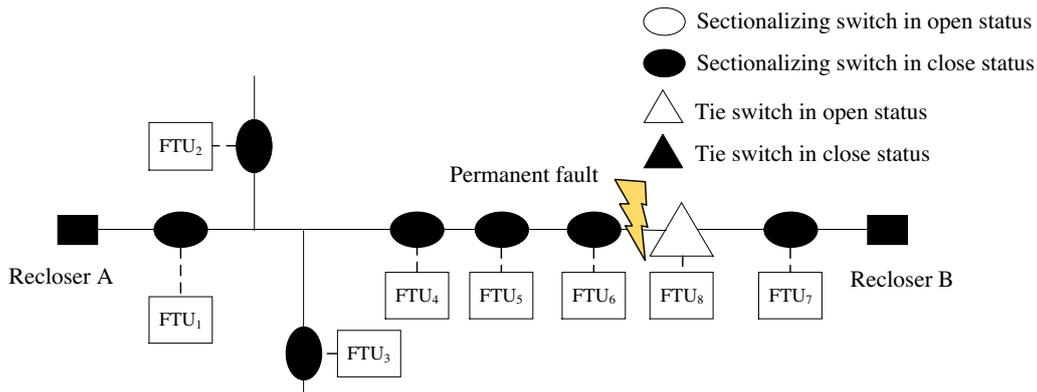
Fig. 2. Single, permanent fault that occurred on the feeder shown in Figure 1
