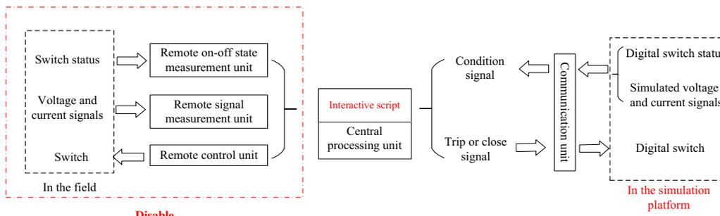
Fig. 9. The operating principle of the embedded interactive script in the FTU
