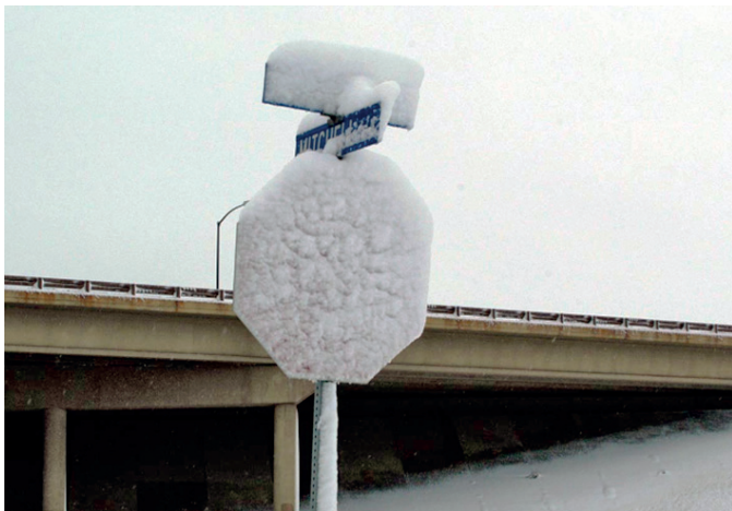
Fig. 14. An example of a road sign that is difficult for vision systems to identify [43], which could easily be recognized using the UWB system
