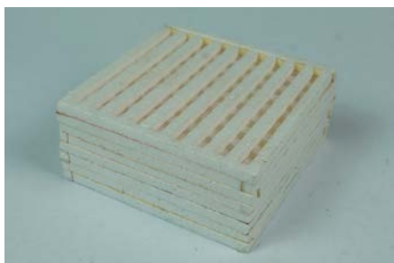
Fig. 11. Glued pattern of porous metal from EPS
