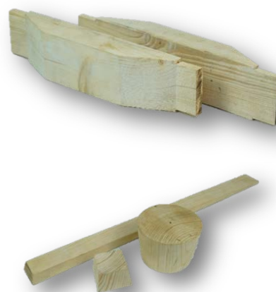
Fig. 8. Wooden pattern of casting and gating system
