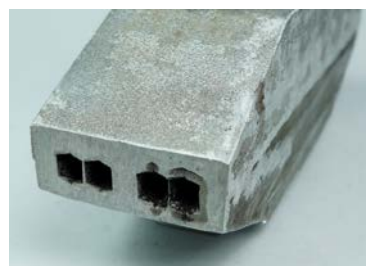
Fig. 10. Detail of the resulting heat exchanger casting
