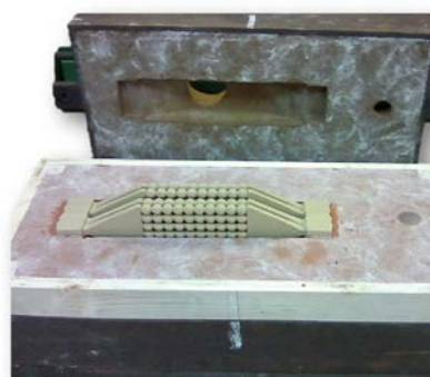
Fig. 9. Mould with inserted preforms
