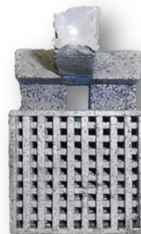
Fig. 12. Cleaned casting, material AlSi10MgMn CSN 424331, top view [22]
