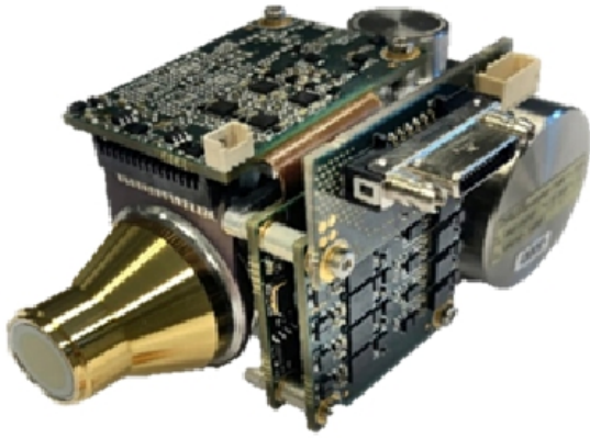
Fig. 12. Oden MW SWaP IDDCA with RM1 cooler in production at IRnova.
