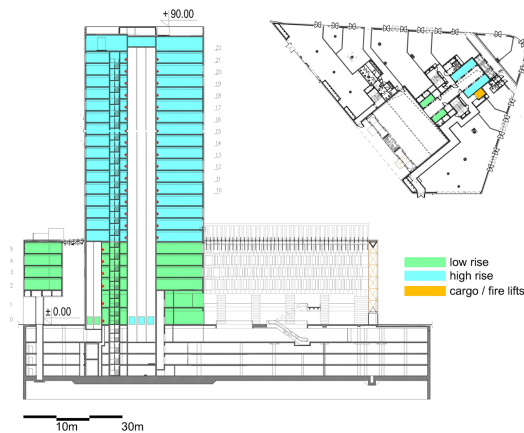
Fig. 1. Cross-section and projection of the ground floor of the building with an indication of the groups of lifts and their scope of operation; source: Author's study
