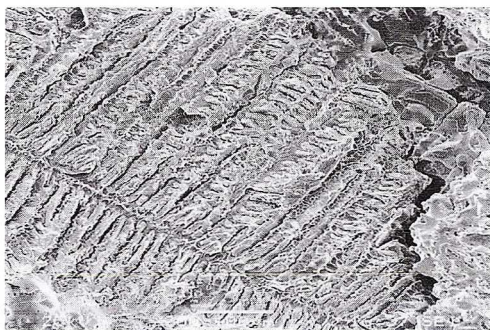
Fig. 9. SEM image of fracture of the die cast Ni 3 Al + 0.05% B material, 200x
