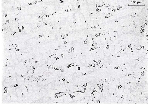
Fig. 23. Microstructure on the surface of Ni 3 Al/(TiB,TiB 2 )/10p composite. Note well visible precipitates of titanium borides, 100x
