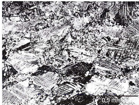
Fig. 19. CuSi3.5 silicon bronze structure at temperature of 600 \text{ }^\circ\text{C} after complex deformation to \epsilon_p=1.7 with strain rate of 0,1 \text{ s}^{-1} and strain amplitude of 0.05
