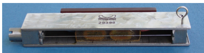
Fig. 2. A VW strain gauge with the ends of the wire directly anchored to the tested object
