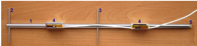
Fig. 9. Prototype differential VW strain gauge. 1 – body housing, 2 – fixed anchor, 3 – movable anchor, 4 – electromagnets, 5 – wire tensioner
