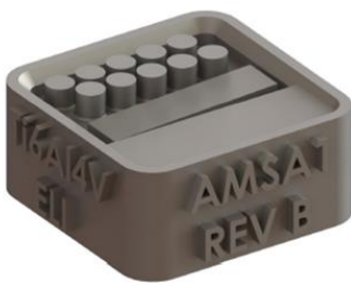
Fig.21. Length artifacts: cylinders, angular surface, flat surface [9]
