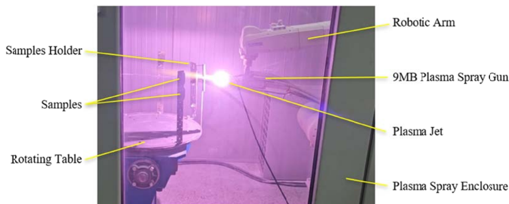
Fig. 2. Aspect during the Plasma Spray procedure
