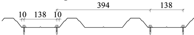
Fig. 2. The arrangement of the sheet-to-purlin fasteners
