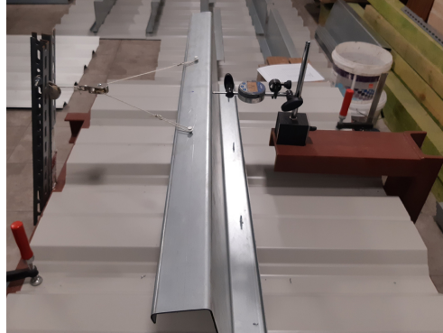
Fig. 4. The 13U specimen under uplift load
