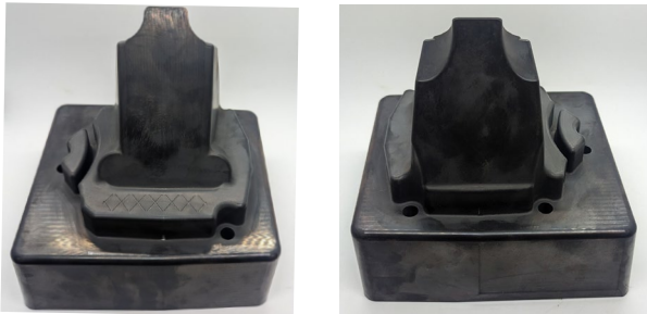
Fig. 2. Gate valve insert at the end of the manufacturing process
