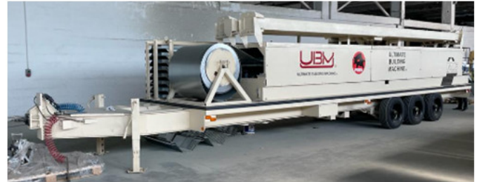
Fig. 3. Prefabrication UBM machine
