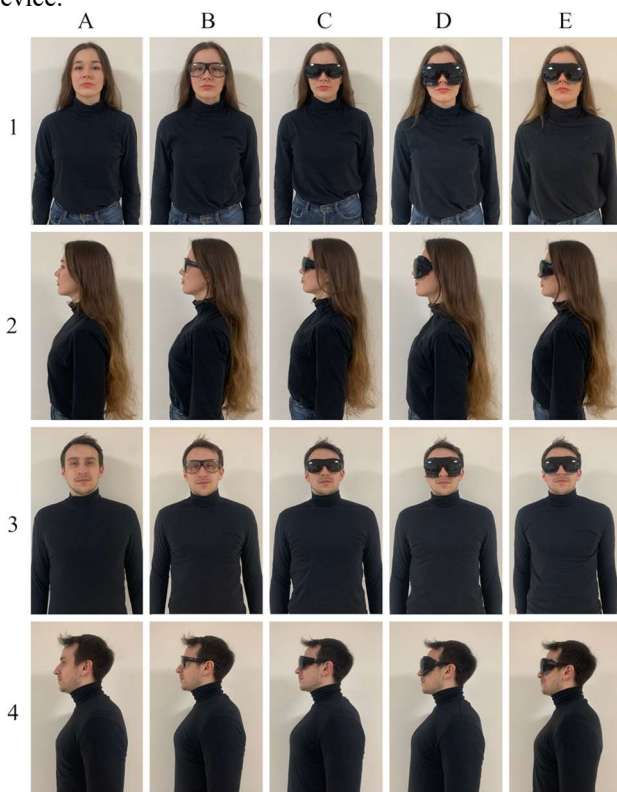
Fig.6. Device Appearance and Analysis of the Perception Difference in a Person Wearing an Eyetracker: A - Without eye tracker, B - With eye tracker, C - With eye tracker and sun visor, D - With eye tracker, sun visor, and the designed shield V1 (first version), E- With eye tracker, sun visor, and the designed shield FV (final version); 1- female silhouette, frontal view, 2- female silhouette, side view, 3- male silhouette, frontal view, 4 - male silhouette, side view
