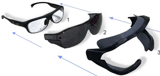
Fig.3. Shield and its mounting mechanism (1. eye-tracker; 2. protective lens [25]; 3. shield FV)
