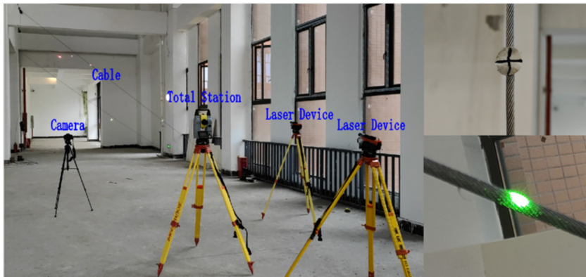
Fig. 10. Experimental site layout and the markers
