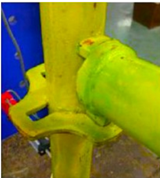
Fig. 3. The socket joint of the scaffold [45]
