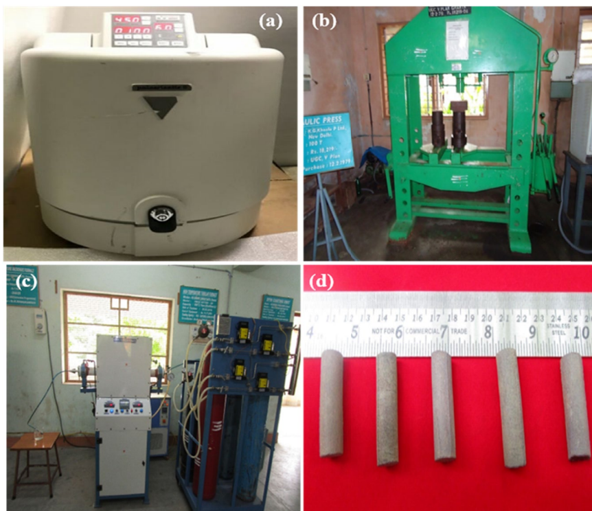
Fig. 2. (a) Ball milling apparatus (Fritch-pulverise-6), (b) Hydraulic pressing machine, (c) High temperature tubular furnace, and (d) Sintered samples
