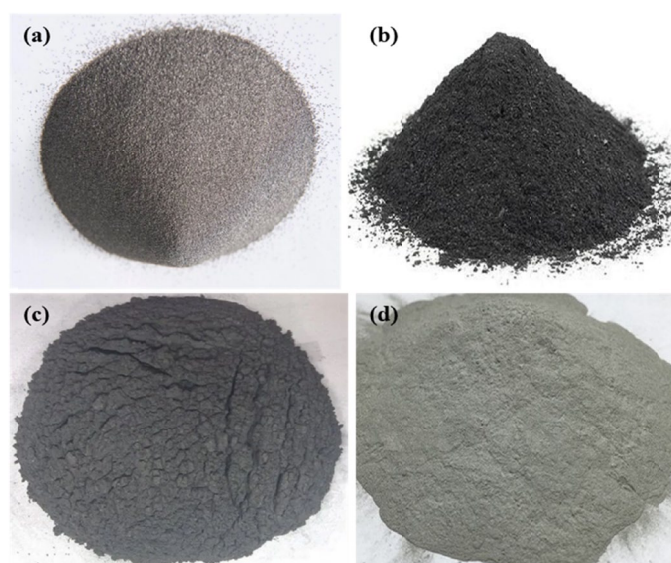
Fig. 1. Raw materials of (a) Titanium, (b) Niobium, (c) zirconium and (d) Tin Powders
