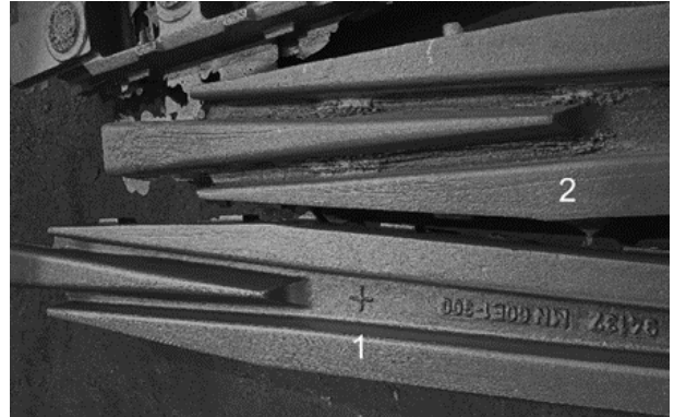
Fig. 1. A view of the running part of Insert R300 frog (net mass 273 kg) cast from manganese cast steel in Huta Małapanew Sp. z o.o. 1 – when moulding sand based on chromite sand in Alphaset technology was used; 2 – when sand based on quartz sand in Alphaset technology was used
