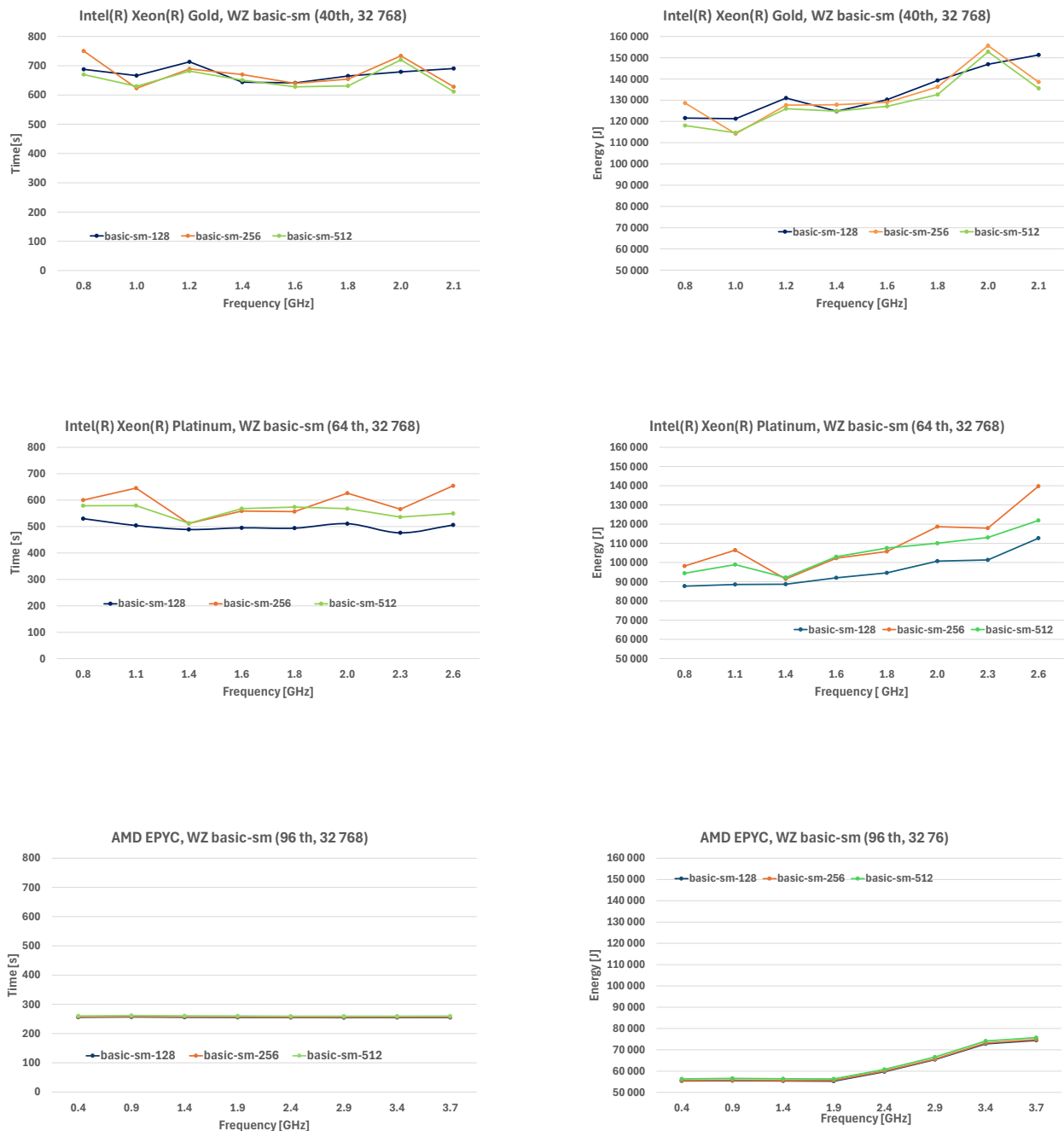
Fig. 5. Runtime and energy consumption of basic-sm for ICC compiler on three computing platforms
