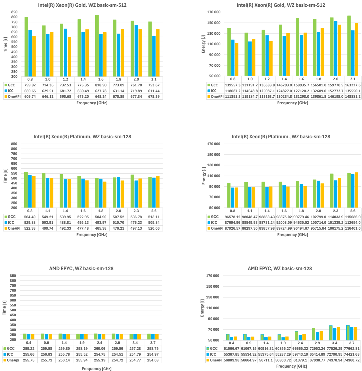
Fig. 6. Runtime and energy consumption of across platforms and compilers for selected block size
