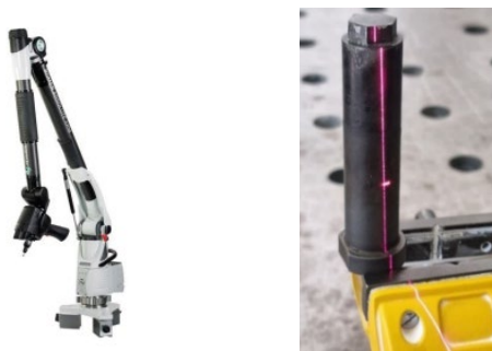
Fig. 2. Example of measurement on the ROMER ABSOLUTE ARM 7525SI laser scanner: a) 3D laser scanner, b) component measurement
