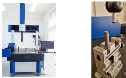
Fig. 3. Example of measurement on the THOME PRÄZISION GmbH coordinate measuring machine: a) coordinate measuring machine, b) component measurement
