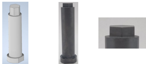
Fig. 1. Example of the analysed component: a) CAD model for additive manufacturing, b) additively manufactured component, c) detail of the working part of the crown
