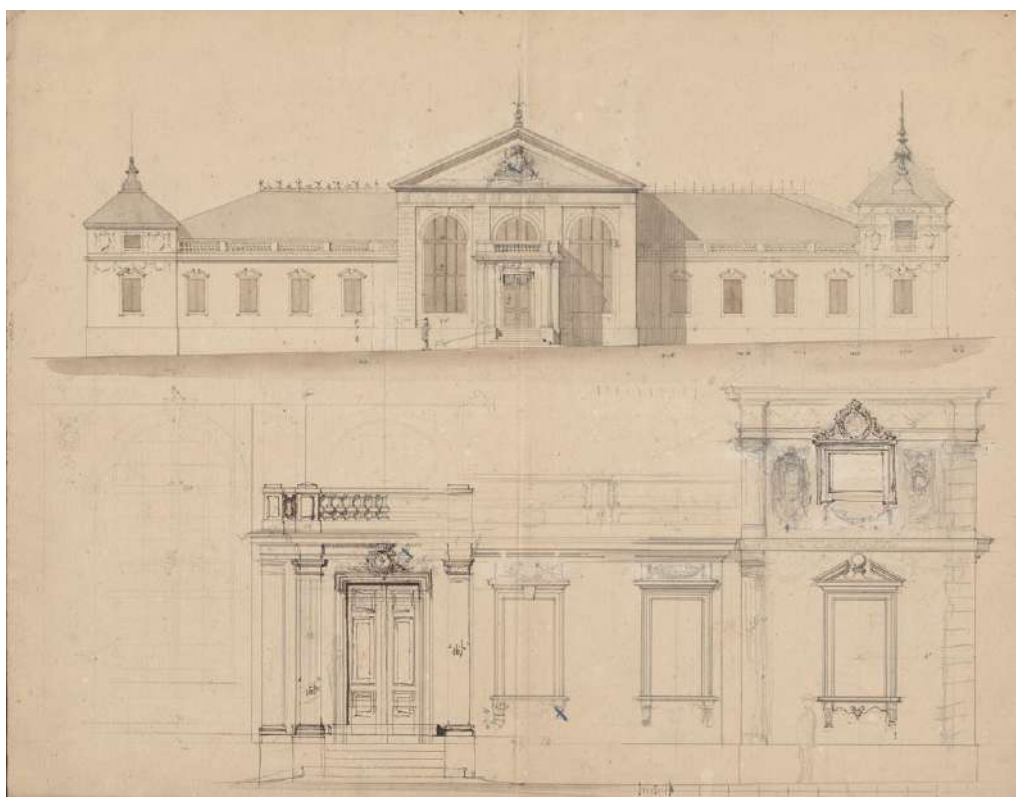
Ill. 7. Design sketches of the reconstruction of the Broel-Plater manor house in Piaseczna, front elevation and details, drawing W Marconi, ca. 1885. MNW Arch., sign.103, vol. II.
