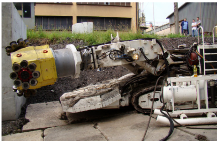
Fig. 23. A view of the KR150 miner arm with a head with disc tools of complex trajectory before field tests
