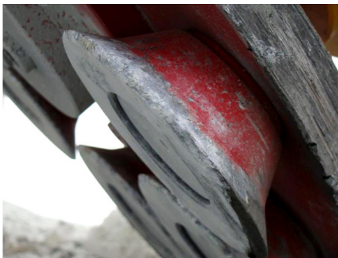
Fig. 26. A view of wear marks on the plate side surface and disc tools
