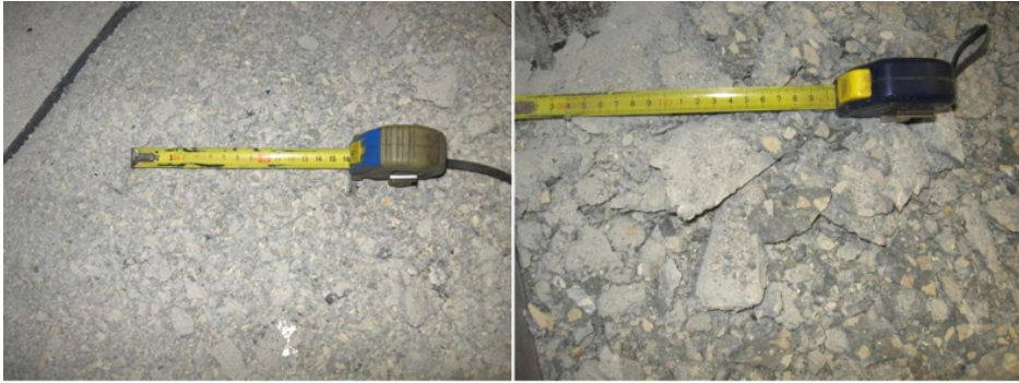
Fig. 17. Graining of the winning obtained during horizontal (left) and vertical (right) mining
