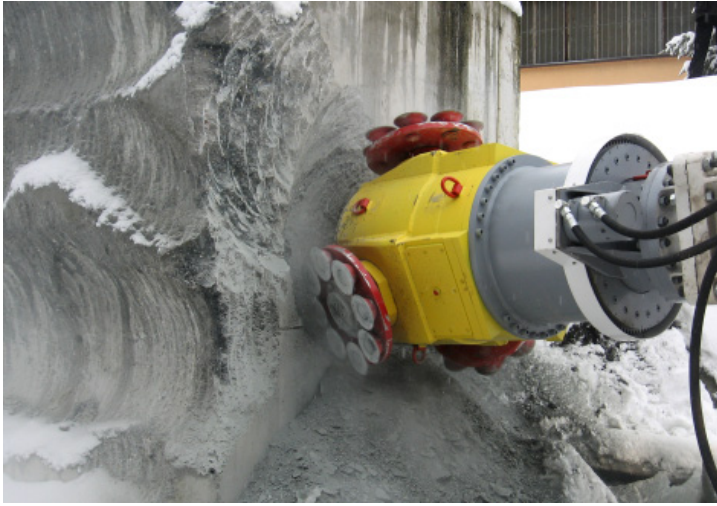
Fig. 24. A view of the KR150 miner with the new head solution with asymmetrical disc tools during one of the field tests
