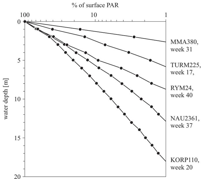
**Figure 2.** Examples of actual PAR attenuation profiles from the surface to the euphotic depth (note: log-linear scales). The sampling station and week are indicated for each profile. MMA380 shows the highest and KORP110 the lowest attenuation in our data
