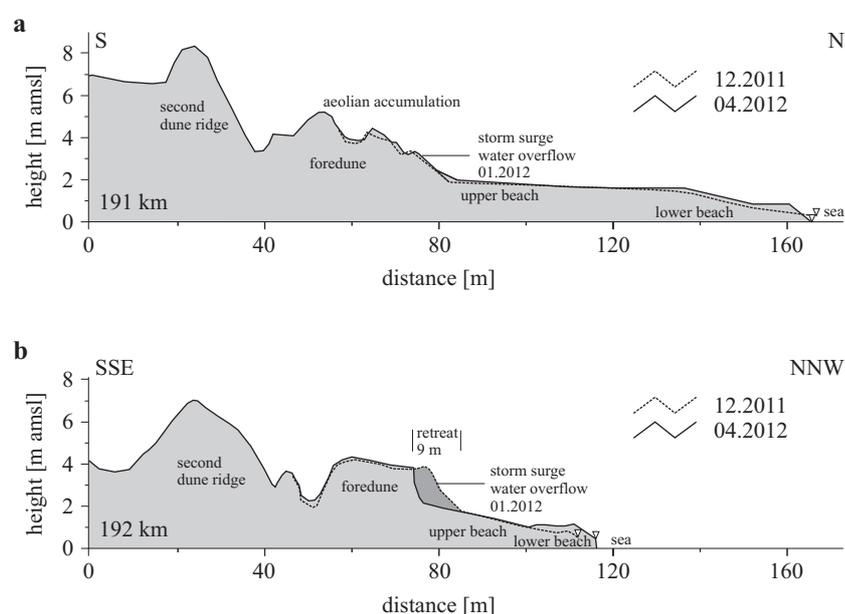
**Figure 8.** Influence of sea level rise during a storm surge (exemplified by the January 2012 storm) on dune relief, Lake Łebsko Sandbar; a) profile resembling a dissipative, low beach: considerable foredune abrasion (191 km), b) profile resembling a reflective, high beach: accumulation prevails (192 km)
