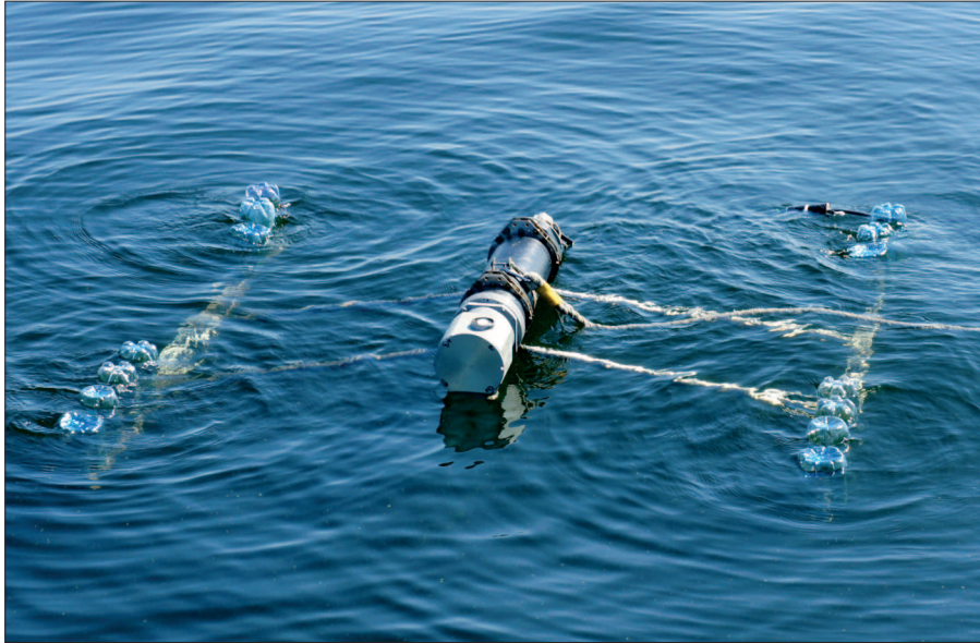
Figure 2. The spectroradiometer used for the measurements
