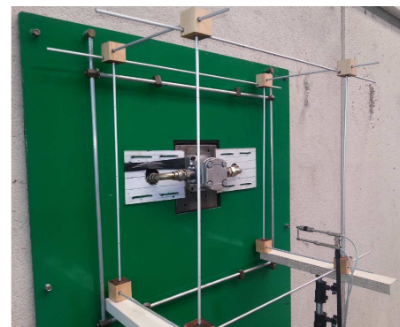
Fig. 8. Sound pressure test (top); surface and sound intensity probe for sound power test (bottom).
