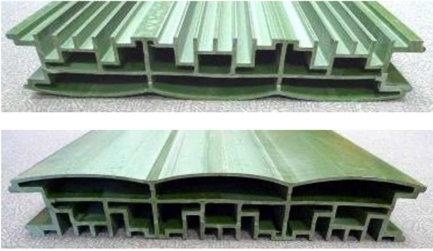
Fig. 2. The prototype of the designed acoustic screen.
