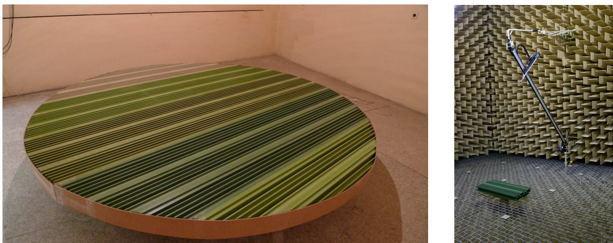
Fig. 7. Tested samples on the measurement setups: the sample used to study sound scattering coefficient (on the left) and the sample used to study sound diffusion coefficient (on the right).
