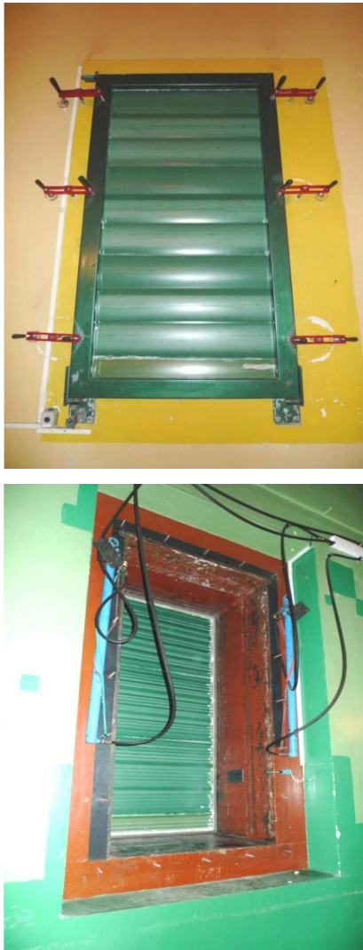
Fig. 10. The sample on the measurement setup intended for determination of elements' sound insulation.
