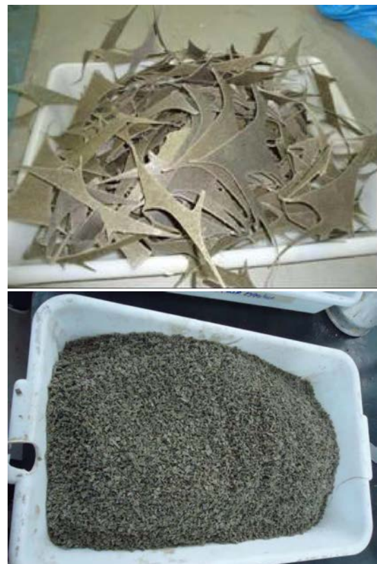
Fig. 2. Counter thermoplastic residue: waste received (top) and after grinding (bottom).
