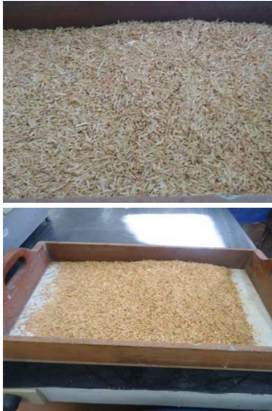
Fig. 3. Rice husk: waste received (top) and after cleaning (bottom).
