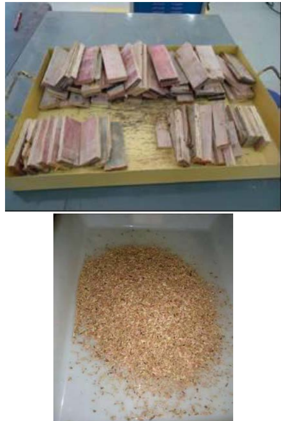
Fig. 1. Residue of plywood resin formwork: cut-off plates (top) and after grinding (bottom).
