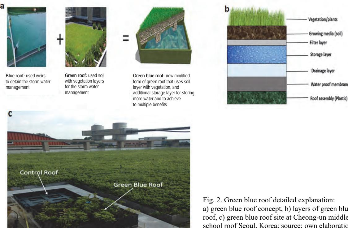
Fig. 2. Green blue roof detailed explanation:
