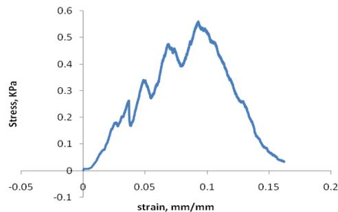
Fig. 3. Stress-strain curve at 22% clay content
