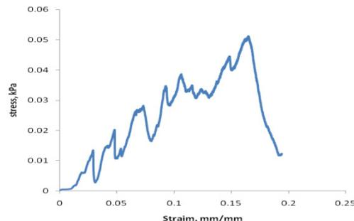
Fig. 5. Stress-strain curve at 30% clay content
