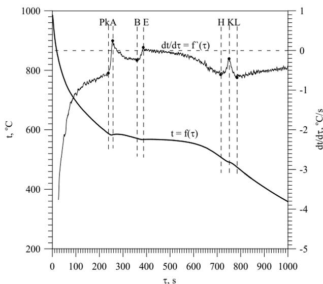
Fig. 2. Representative DTA curves of 226 silumin
