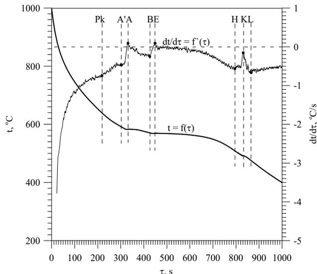
Fig. 3. Representative DTA curves of silumin containing approximately 0.2% Cr and W
