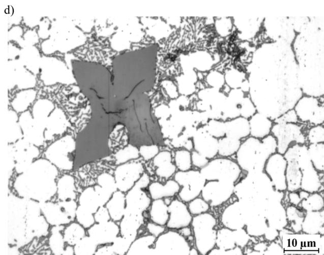
Fig. 5 (a-d). The microstructure of die casting made of the tested silumin containing Cr and W approximately: a – 0.1%, b – 0.2%, c – 0.3% i d – 0.4%:  $\alpha$ ,  $\alpha + \text{Al}_6\text{Fe}_3\text{Si}_2 + \beta$ ,  $\alpha + \text{Al}_2\text{Cu} + \text{AlSiCuFeMgMnNiCrW} + \beta$
