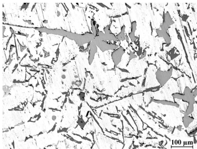
Fig. 4. The microstructure of silumin containing approximately 0.4% Cr and W obtained in the DTA sampler:  $\alpha$ ,  $\alpha + \text{Al}_9\text{Fe}_3\text{Si}_2 + \beta$ ,  $\alpha + \text{Al}_2\text{Cu} + \text{AlSiCuFeMgMnNi} + \beta$
