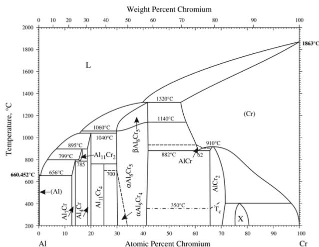
Fig. 1. Aluminum-chromium phase diagram [16]
