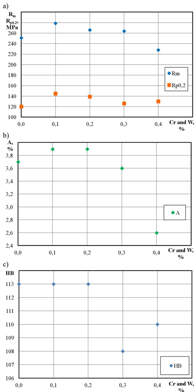
Fig. 6 (a-c). The mechanical properties of the tested silumin, without and with the addition of Cr and W: a –  $R_m$  and  $R_{p0,2}$ ; b – A; c – HB
