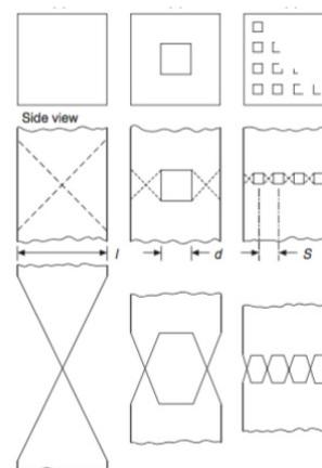
Fig. 7. Simple ductile failure model [2]
