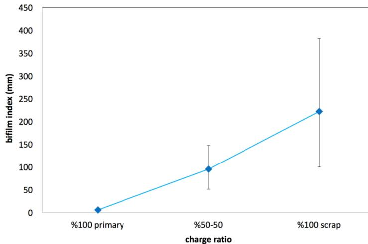
Fig. 4. Bifilm index of different charges
