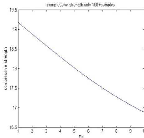
Fig. 6. Compressive strength (kg/cm<sup>2</sup>) vs Ph
