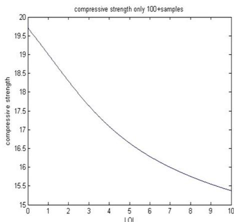
Fig. 7. Compressive strength (kg/cm<sup>2</sup>) vs LOI
