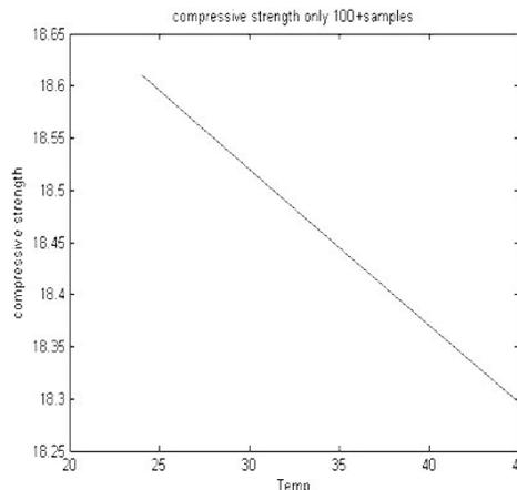
Fig. 5. Compressive strength (kg/cm<sup>2</sup>) vs Temperature
