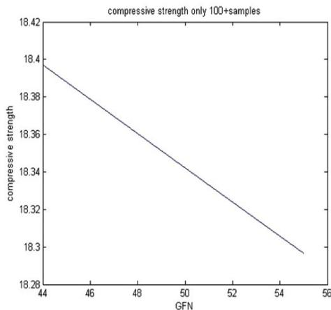
Fig. 4. Compressive strength (kg/cm<sup>2</sup>) vs GFN
