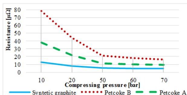
Fig. 4. The change of the resistance due to the applied compressing pressure for selected carburizers
