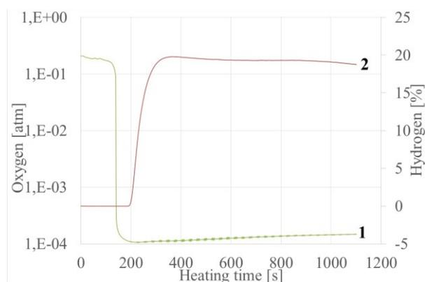
Fig. 9. Hydrogen and oxygen content in emitted gases: 1 - oxygen, 2 – hydrogen
