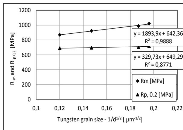
Fig. 7. The relationship between tensile and yield strength and the value of  $1/d^{1/2}$
