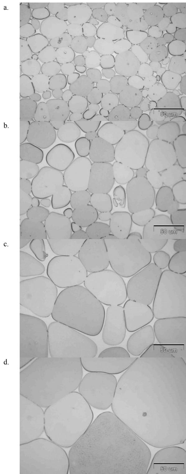
Fig. 3. The microstructure of THA after different number of sintering cycles: a - 1 cycle, b - 2 cycle, c - 5 cycles and d - 15 cycles
