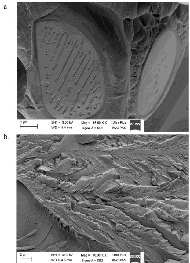
Fig. 5. The morphology of fracture surface structure of specimen after: a- one and b – 15 sintering cycles
