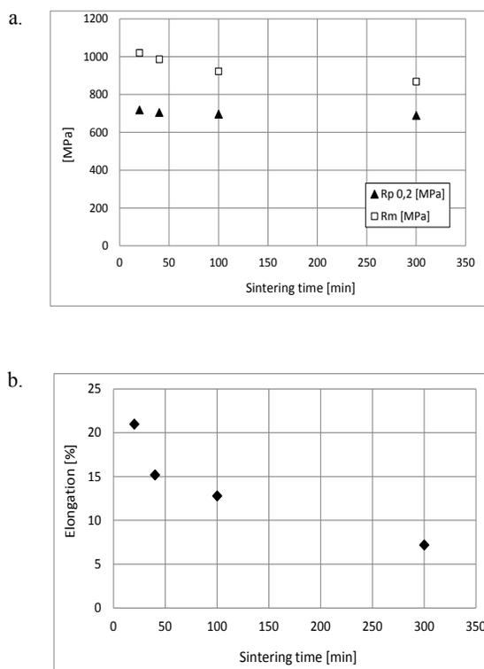
Fig. 2. The results of tensile test as function of sintering cycles:
