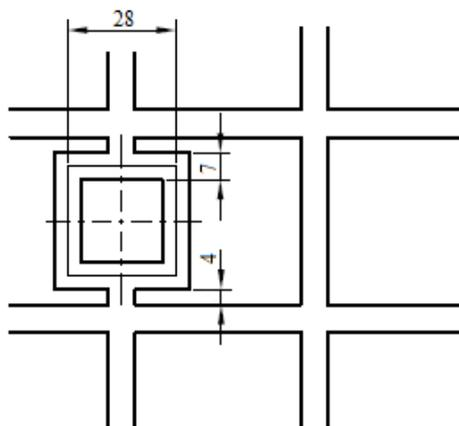
Fig. 2. The shape and dimensions of the flexible segment
