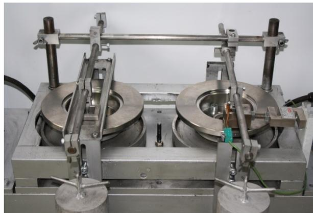
Fig. 1. A view of the set-up for brake disc abrasion resistance test
