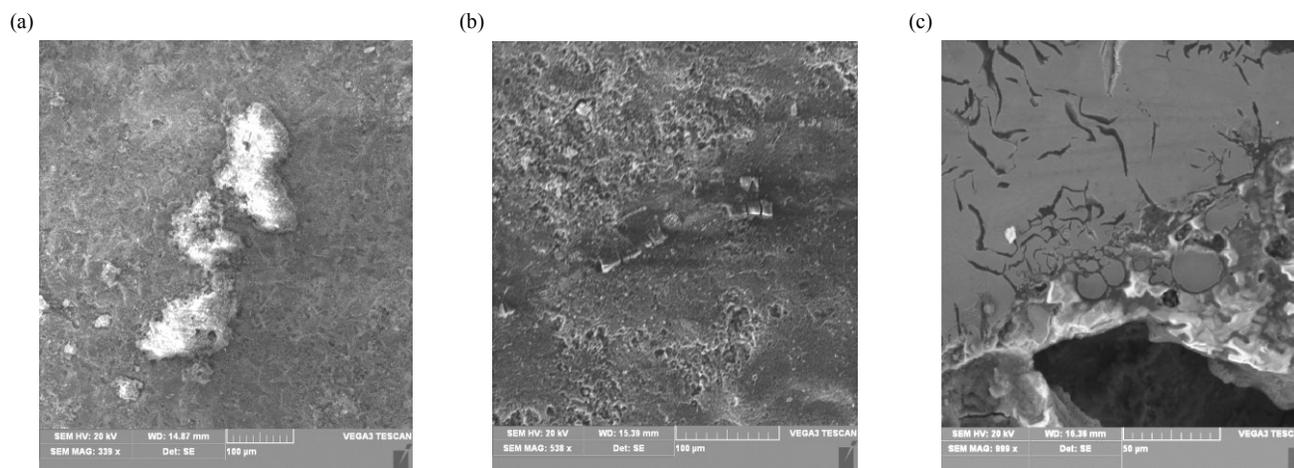
Fig. 2. An example view of a thin-wall casting non-conformity: (a), (b) on wall surface; (c) a view in transverse section — a cluster of cold shots at the casting surface
