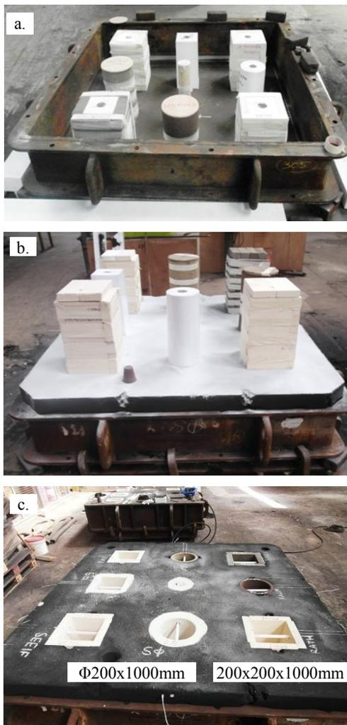
Fig. 1. Selected stages of producing a mould containing tested materials: iso-exo sleeves and insulating bricks. a – patterns with assembled materials – lower (drag) mould, b – preparation of upper (cope) mould, c – mould instrumentation
