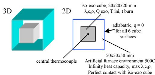
Fig. 10. Schematic geometries (3D and 2D) used in simulation tests
