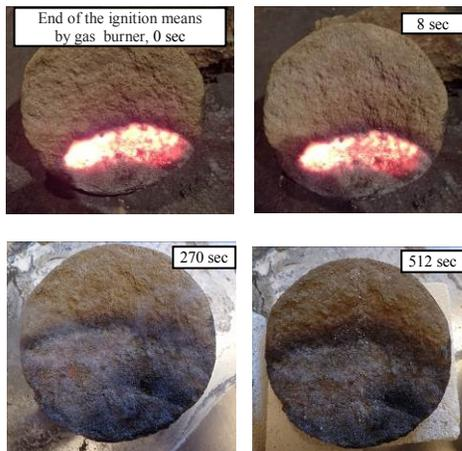
Fig. 6. Ignition test of an iso-exo material by gas burning heating. The initiated exo reaction extinguishes after about 500 s
