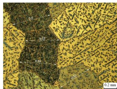
Fig. 6. Brass microstructure in point No. 3
