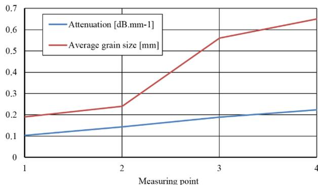
Fig. 8. Attenuation and average grain size in measuring points
