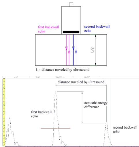
Fig. 3. The principle of attenuation determining
