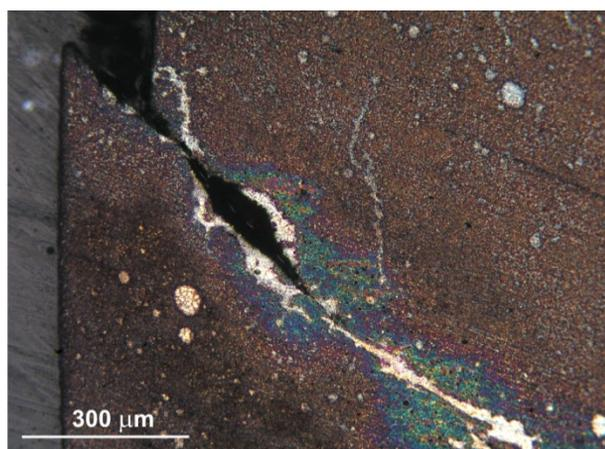
Fig. 7. The microstructure of the AC-44200-40 vol. % Al<sub>2</sub>O<sub>3</sub> with the slip crack after deformation. Test temperature: 150°C
