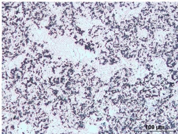
Fig. 3. Microstructure of the composite material EN AC-44200 - 20% vol.  $\alpha$ - $\text{Al}_2\text{O}_3$  particles
