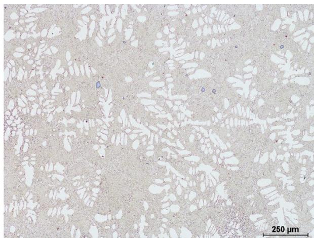
Fig. 1. Microstructure of the matrix alloy EN AC-44200
