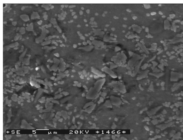
Fig. 13. SEM of the fracture with the delamination of EN AC-44200-20 vol. % of  $\text{Al}_2\text{O}_3$  material in the mid-section of the sample. Test temperature 20°C
