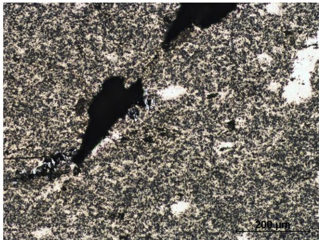
Fig. 10. The cracks of a composite material EN AC-44200-30 vol. %  $\text{Al}_2\text{O}_3$ . Test temperature 150°C
