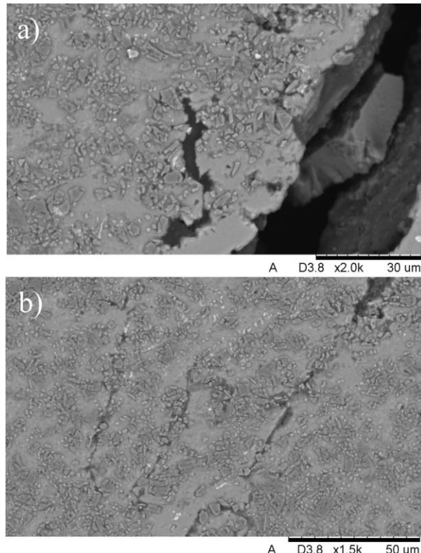
Fig. 12. SEM of a fracture of sample: a) material EN AC-44200-30 vol. %  $\text{Al}_2\text{O}_3$ , b) material EN AC-44200-40 vol. %  $\text{Al}_2\text{O}_3$ . Test temperature 20°C
