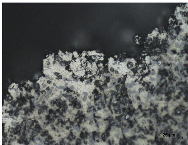
Fig. 9. The deformed composite EN AC-44200-20 vol. % Al<sub>2</sub>O<sub>3</sub> material in the vicinity of the slip crack. Test temperature: 20°C
