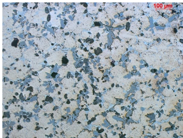
Fig. 4. Microstructure of the weight alloy, LM
