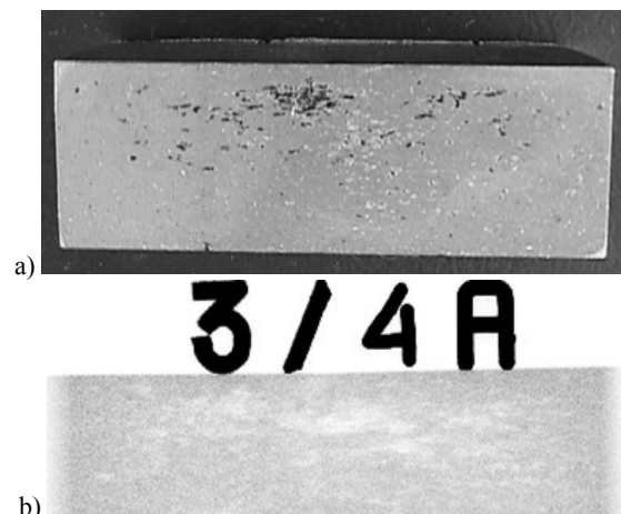
Fig. 4. Shrinkage porosity – reinforcement: aluminosilicate fibres, matrix: AlSi11; a) composite structure (macroscopic tests), b) the same composite – a digital image from a radiogram (X-ray defectoscopy)
