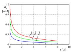
Fig. 7. Changes in coaxial MCG tubes' resistance taking into account the skin effect: 1 – resistance of both tubes, 2 – resistance of the internal tube, 3 – resistance of the external tube
