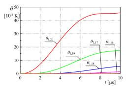
Fig. 9. Temperature rise distribution of the internal tube in node  $r_n = 0.5D_1 + n\Delta_1$ , where  $\Delta_1 = 0.5(D_2 - D_1)/20$
