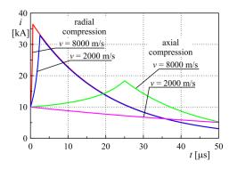
Fig. 13. Current *i* for an MCG with axial and radial compression for a = 0.2 m,  $D_3 = 2$  cm,  $D_2 = 1$  cm
