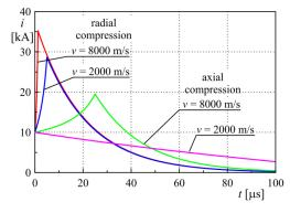
Fig. 11. Current *i* for an MCG with axial and radial compression for a = 0.2 m,  $D_3 = 4$  cm,  $D_2 = 2$  cm
