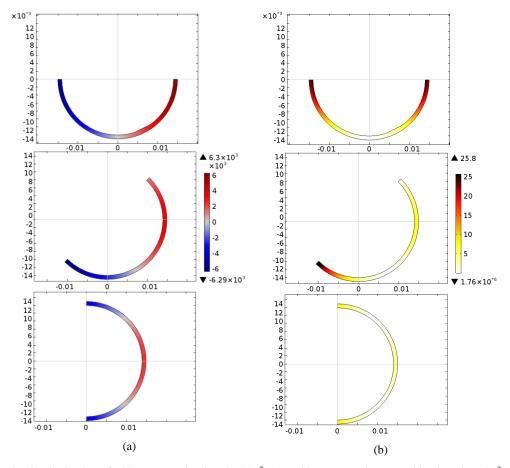
Fig. 4. Distribution of eddy currents density j in A/m<sup>2</sup>: (a) and heat generation caused by them in W/m<sup>3</sup>; (b) shown on the cross-section of the split shell with angle  $\beta$  of (top to bottom) 0°, 45°, 90°
