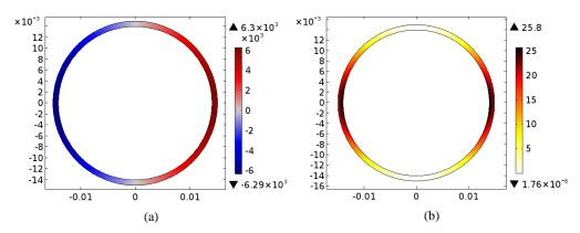
Fig. 3. Distribution of eddy currents density j in A/m<sup>2</sup>: (a) and heat generation caused by them in W/m<sup>3</sup>; (b) shown on the cross-section of the shell
