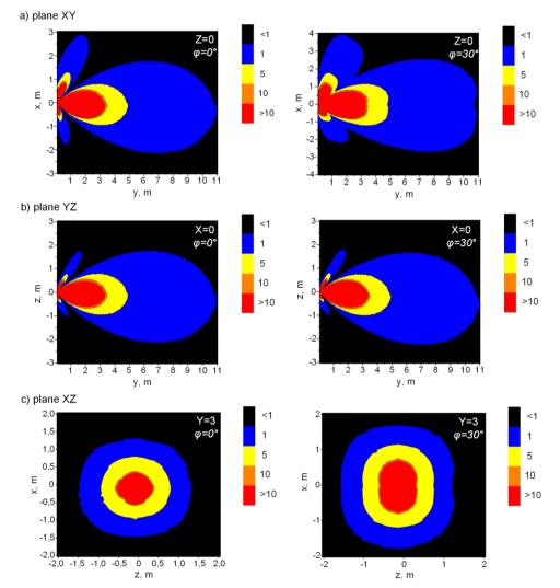
Fig. 8. Cross section of the interrogation zone done in coordinate plane: a) XY; b) YZ; c) XZ
