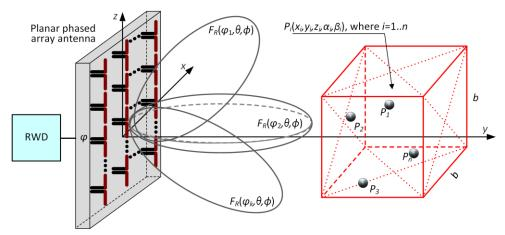
Fig. 2. Problem of objects identification in the UHF RFID systems with RWD planar phased array antenna
