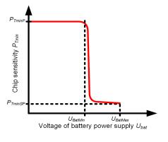
Fig. 4. Generalized curve of sensitivity for passive and semi-passive chip
