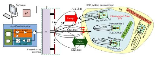
Fig. 1. Anti-collision UHF RFID system with phased array antenna
