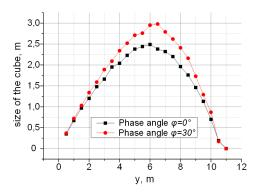
Fig. 7. The sample results of the size of the interrogation zone determined in calculation process for:  $\phi=0^\circ$  and  $\phi=30^\circ$
